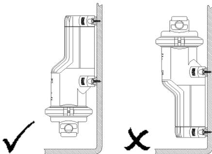
When mounting, position the pump on the intended surface and work-out the best angles for the hose, then mark the 4 hole positions using the pump feet. The pump head may be rotated to suit the hose connections, this is done by loosening the two screws that hold the clamping rings, and rotating the pump head. Once you have marked the position for the four mounting feet, drill four pilot holes of 3.2mm ( $1/8$ ""). Use the four No.8 self tappers and washers to
