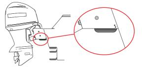
The transducer transom bracket can be mounted inside or outside of the jackplate by drilling through the jackplate and then running bolts through the hinge hole in the side of the bracket into the jackplate. The illustration above shows the transom bracket mounted inside the jackplate.
