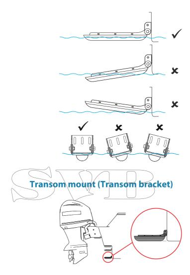
The transducer can be mounted on a transom bracket. With this mounting option the transducer can be in the water when you are on plane, or can be mounted so it is only in the water when you are moving at trolling speed.
