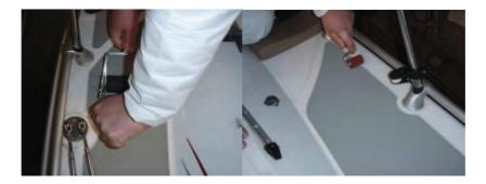
If there are air bubbles, remove them with the hypodermic needle of a syringe (do not use a cutter). Do not peel off large parts of the covering from the support to remove a bubble, or the adhesive film could be ruined and the TBS panel would become unusable.
