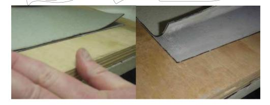
e) To make sure no air is left under the covering, you have to roll very hard on the covering and the edge, following the furrows made by the scraper, so that the air can evacuate correctly without creating air bubbles or surpluses of adhesive.
