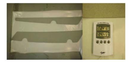
a) Dust with a dry cloth and remove the grease with acetone. Do not use White Spirit because it would leave a greasy film. Leave the solvent to evaporate (30 minutes).
