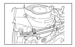
12. Remove the bolts securing the recoil starter in place.
