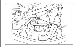
To maintain a strong spark, you should clean and adjust the plugs at the intervals shown in the maintenance chart. Remove carbon deposits from the spark plugs using a small wire brush or spark plug cleaner, and adjust the gap according to the following chart:
