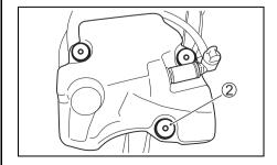
11. Disconnect the throttle cables from clamp  $\Im$ .
