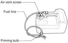
SEPARATE FUEL TANK (Optional parts for DF5A/DF6A)
