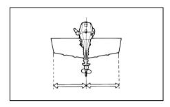
Install 8 mm bolts, washers, lock washers and nuts, as illustrated and tighten the bolts sequentially. Be sure to seal the holes with sealant to prevent water leakage.
