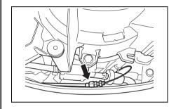
Remove the bolts securing the fuel tank in place.
