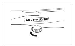
20. Twist the air-vent screw on the fuel tank cap counterclockwise to open the vent.
