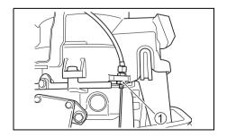
Separate the end of cable from the recoil starter.
