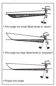
Make a test run in the boat to determine if the trim angle needs to be adjusted.
