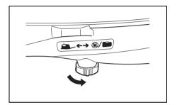
4. Tighten the air-vent screw on fuel filler cap.
