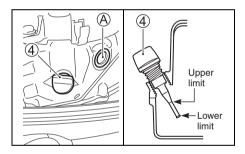
The oil on the filler cap (dipstick) should be between the upper and lower limits shown on the filler cap.
