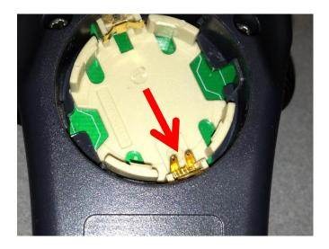
These two pins need to be in contact with the underside the battery. They should not be bent upward, in contact with the side of the battery as shown below.
