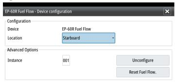
'Unconfigure' is for defaulting the device clearing all user settings, and 'Reset Fuel Flow' will restore only the 'Fuel K-Value' setting, if set in 'Calibrate'. Only Navico devices can be reset.
