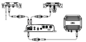
→ Note: the NSO evo2 uses RJ45 sockets, so the RJ45 to 5-pin adaptor is needed for connection to 5-pin (orange plug) ethernet cables. One is supplied with unit.
