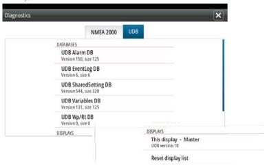
The 'Reset Display List' can be used to refresh the list of connected displays and their UDB version.
