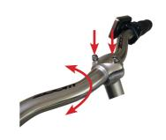
4. Make sure that the display's cable joint attached to the headtube is screwed down tightly for it to be properly water-tight.
