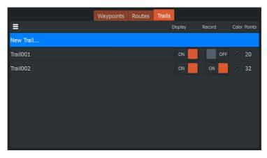
From the factory, the system is set to automatically track and draw the vessel's movement on the panel. The system continues to record the trail until the length reaches the maximum points, and then automatically begins overwriting the oldest points.
