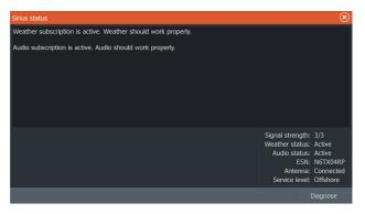
The status panel shows signal strength is indicated as 1/3 (weak), 2/3 (good) or 3/3 (preferred). It also includes antenna status, service level, and the electronic serial number for the weather module.
