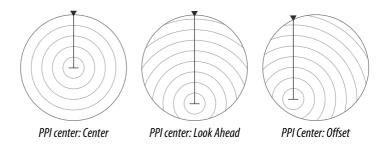
You return the antenna center to PPI center by using the offset option in the View menu.
