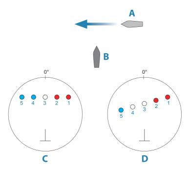
The examples show the target movement (1-5) over 5 radar scans with the radar in relative motion mode.
