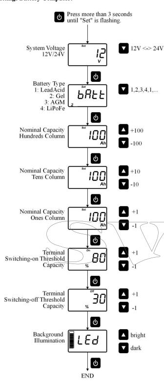
The menu for settings is called by pressing and holding button 3 for more than 3 seconds. The buttons 1 and 2 are used to set the values. In the menu, the button 3 is used to save the setting and to jump to the next menu item.
