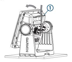
2 Tilt the device forward, and lift it out of the cradle.
