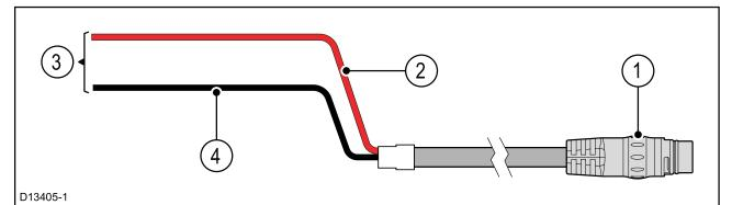
**Note:** A Y-adapter cable (part number A80308) is available for existing installations that already use a combined power/data cable from a Digital or HD Color Radome. The Y-adapter splits the existing combined cable into the separate data and power connectors used by the scanner.
