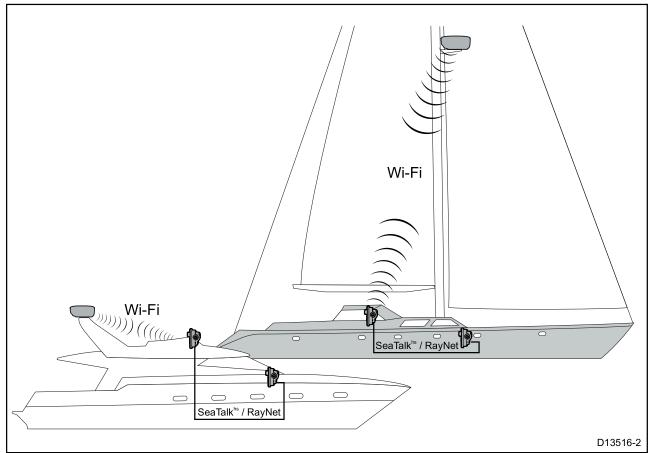
In systems with multiple MFDs, the Radar should be connected to the MFDs that are located closest to it, or to the MFDs with the clearest line of sight to the Radar.
