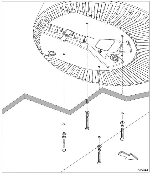
7. Tighten the bolts to a torque of 15 Nm (133 ft lbf).
