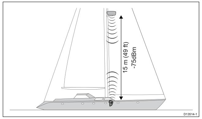
In the example above the maximum distance with acceptable Wi-Fi performance is 15 m (49 ft), due to the heavy fiberglass coach roof that the signal has to pass through.
