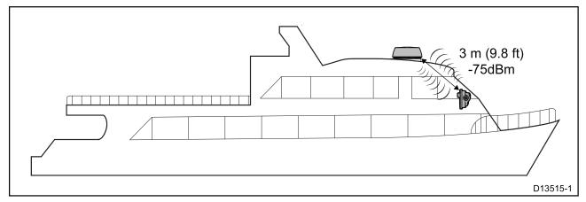
In the example above the maximum distance with acceptable Wi-Fi performance is 3 m (9.8 ft), due to the metal roof that the signal has to pass through.
