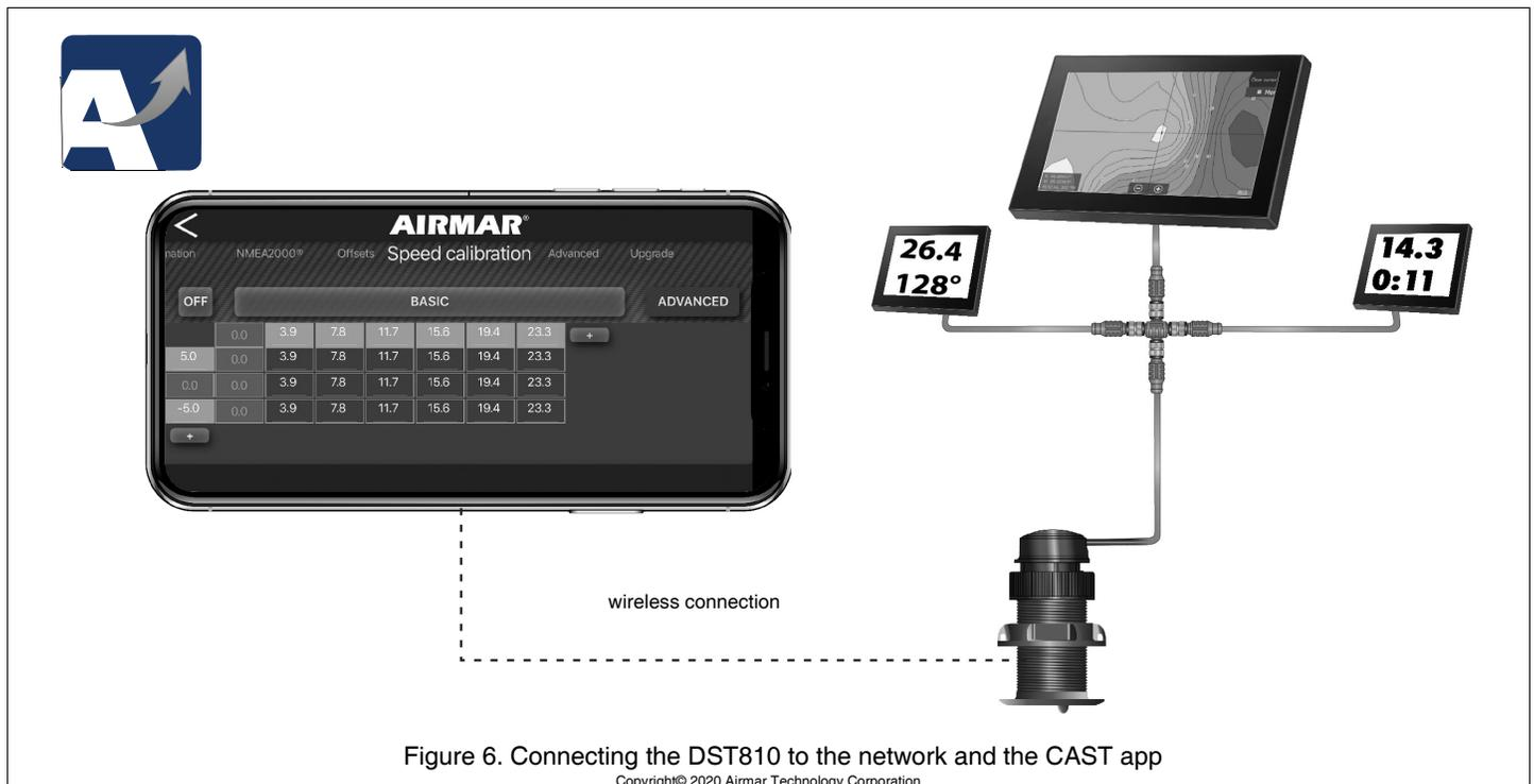
Figure 6. Connecting the DST810 to the network and the CAST app
