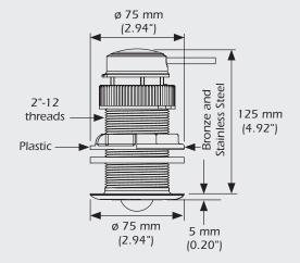
Airmar's innovative housing design incorporates a self-closing valve to minimize water flow into boat when the insert is removed.
