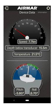
Calibrate basic or heel compensated speeds
