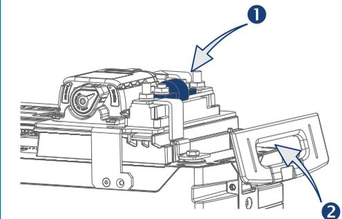
Remove the clear fuse cover and install the T-fuse (1). Place the cover back on the fuse holder. Close the side handle as much as possible (2). It will not close completely.
