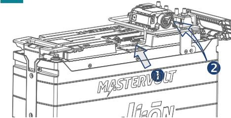
Put the Battery Safety Connector back in place (1). On the ML Switch, set the safety relay knob to "LOCK OFF" (2). Check all wiring and connections.
