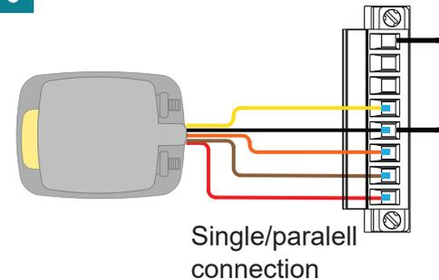
On the Battery Safety Connector, move the jumper wire to pins 4 & 8. Connect the ML Switch wires to the Battery Safety Connector according to the detailed figures in the user manual of the MLI Ultra.
