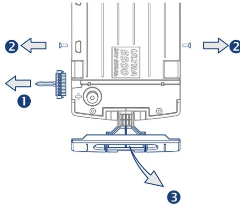
From the MLI Ultra, remove the Battery Safety Connector (1) and on either side the bolt closest to the positive terminal (2). Tilt the positive (right) side handle (3).
