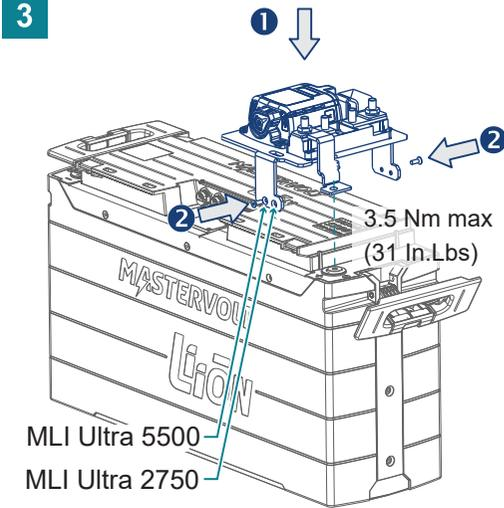
Place the bracket over the MLI Ultra (1), aligning the bracket holes with the holes of the bolts. Tighten the bolts back in place (2).
