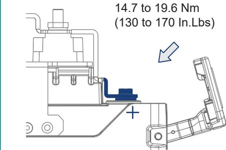
Secure the busbar conductor on the bracket to the positive terminal of the MLI Ultra.
